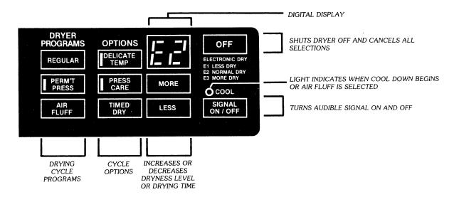
The right portion of the computer touch control panel programs the dryer. The dryer selections can be seen at a glance. Red indicators light up in the pads of the programmed selections.
